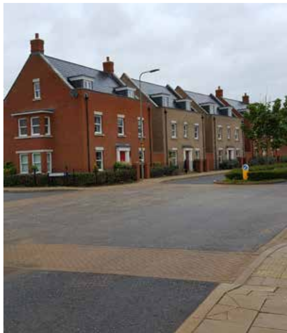
Tarmac with subtly coloured block paving indicating informal pedestrian crossings, South West Bicester
